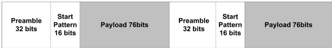
Figure 3.12: Two concatenated packets structure of a rolling code for Chamberlain
