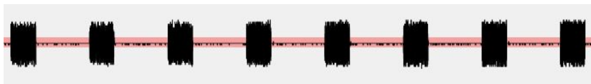
Figure 3.9: A recorded signal contains eight packets
