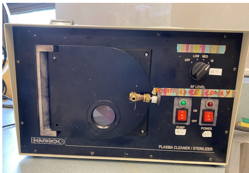
Figure 2.2: Harrick (PDC-002) plasma cleaner used for sterilizing the samples as well as for plasma etching.
