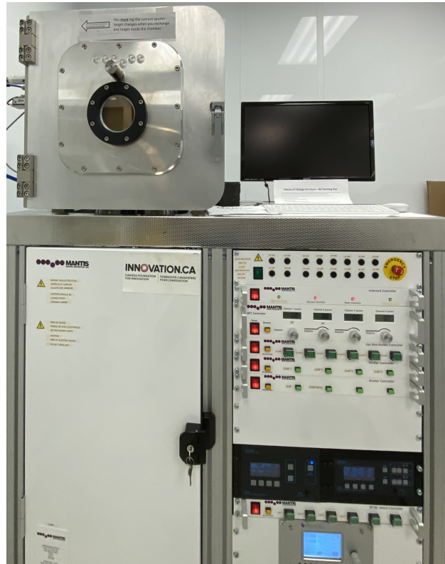
Figure 2.3: Mantis QUBE sputter deposition system
