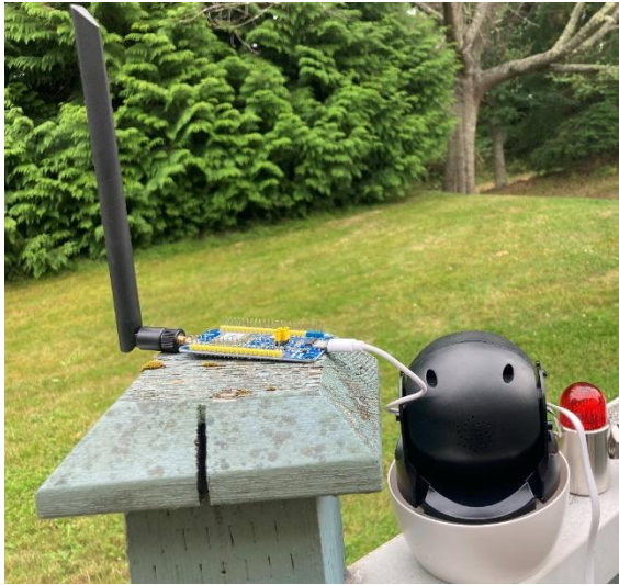
(a) End node with antenna connecting with Camera-embedded system
