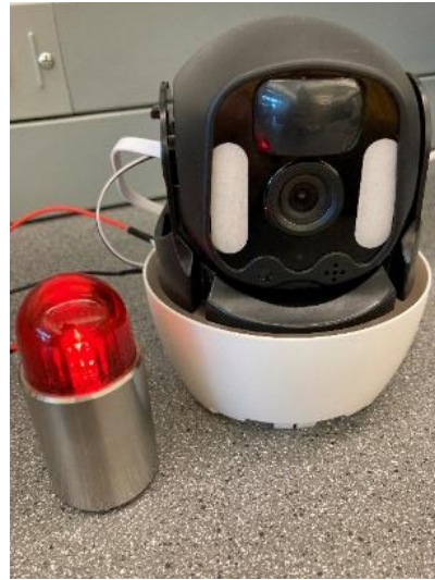
(b) Camera-embedded system with alarm
