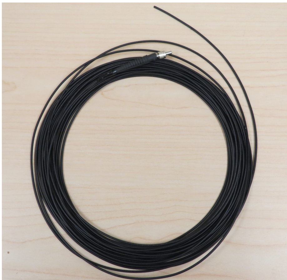
Figure 4.7: Picture of the 15 m long polyethylene cord that protects the polystyrene scintillator and optical fiber, displaying the silver input connector (connects to photosensor module) with the scintillator housed within a 2 mm depth located at the opposite end of the cord.
