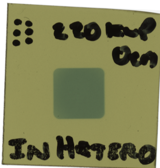
Figure 4.10: Picture of EBT3 film exposed to a 10 x 10 mm 2 radiation field with irradiation notes written on film with Sharpie pen.
