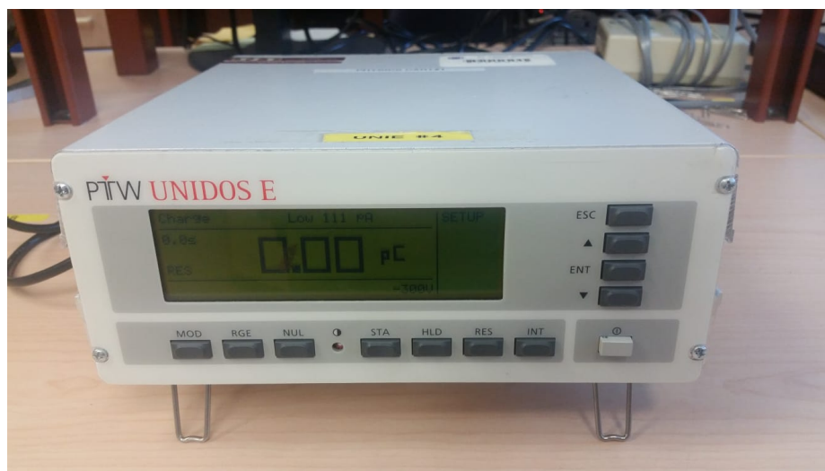
Figure 4.9: Picture of the PTW UNIDOS E electrometer. Photo credit: Dr. Samantha Van Nest.
