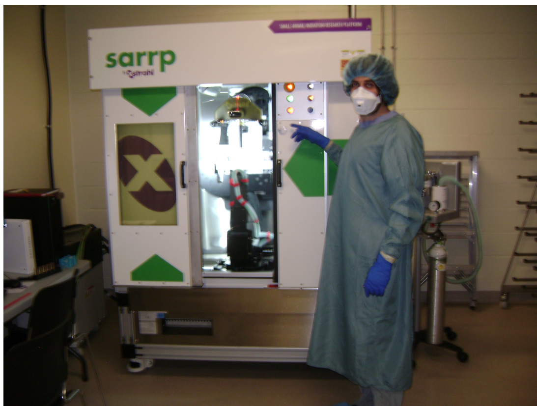
Figure 4.1: Xstrahl SARRP small animal irradiator, with cabinet door open.
