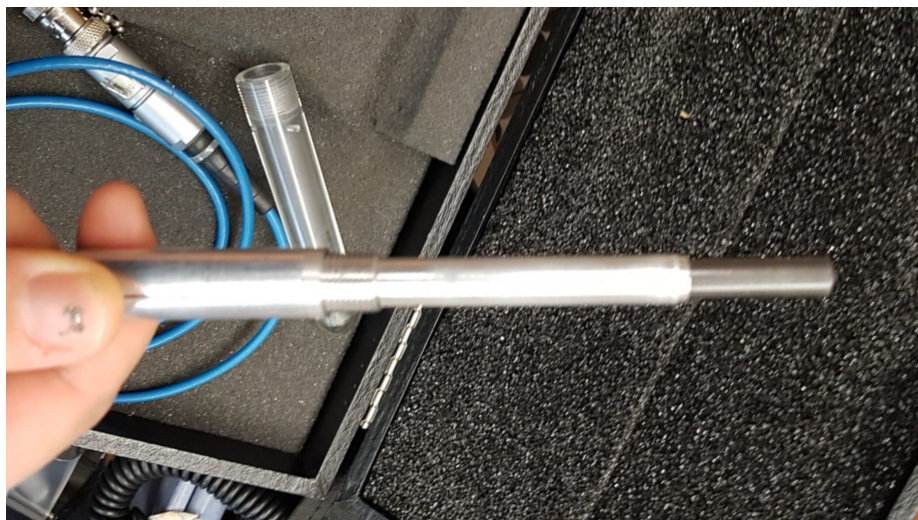
Figure 4.5: Picture of the PTW 31013 farmer-type ionization chamber. Photo credit: Chelsea Dunning.
