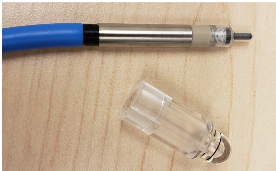
Figure 4.6: Picture of the PTW 31014 PinPoint ionization chamber next to buildup cap.
