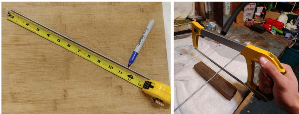
Figure A.19: Cutting of the metal rods.
