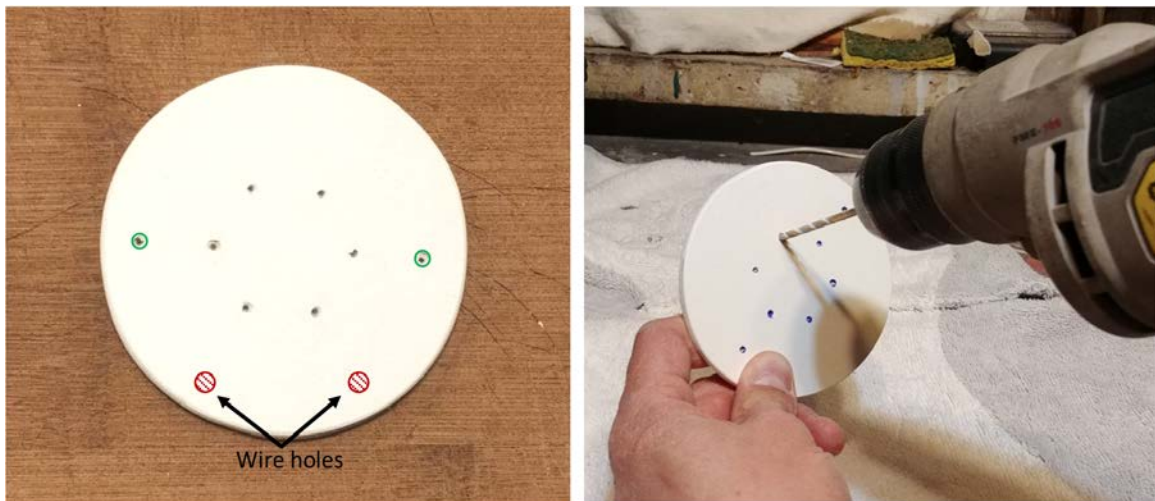
Figure A.17: Drilling of the holes on the discs.
