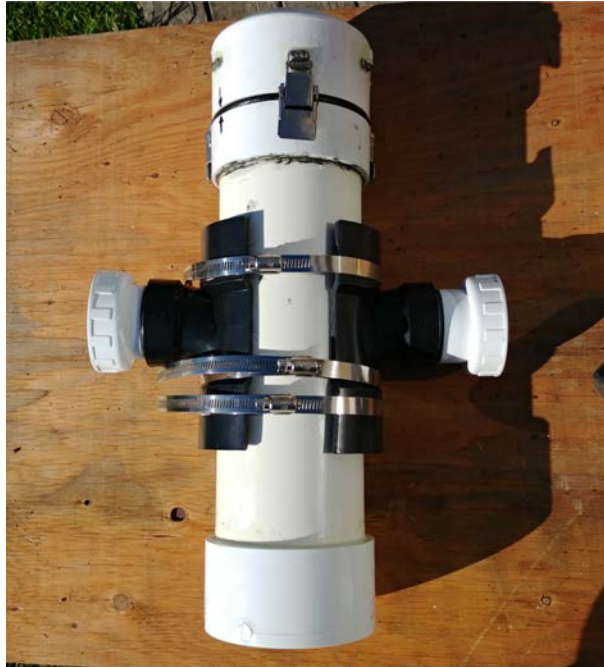
Figure A.31: Installation of PVC attachments to the pressure housing of the Fishcam.
