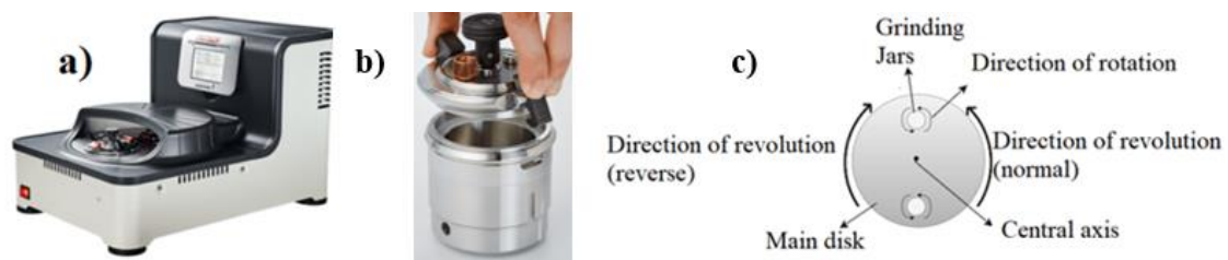
Figure 2. 5. (a) Fritsch Pulverisette 7 Micro Mill premium line. (b) Grinding jar (c) Overall layout of planetary disk of Fritsch Pulverisette 7.
