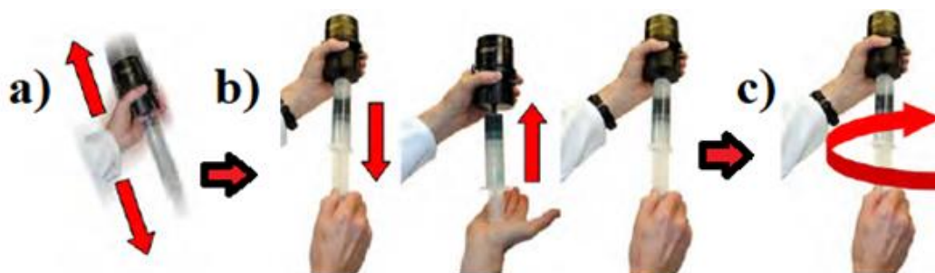
Figure 2.7. Steps for extraction (a) shaking bowl containing suspension vertically for 3-5 times (b) Pull-push suspension containing syringe for 2-5 times (c) extract suspension slowly from grinding bowl.
