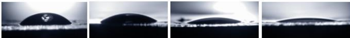
Figure 3.11. (a) Sequence of water drop images on \text{TiSi}_2 films (coated on glass substrates) vs. heating time at 400^\circ\text{C} under argon atmosphere (grinding in EG at 400 rpm for 180 minutes). From left to right: No heating ( \text{CA} = 37.7 \pm 1^\circ ); 30 min ( \text{CA} = 23.8 \pm 1.5^\circ ); 60 min ( \text{CA} = 17.3 \pm 1^\circ ) and 180 min ( \text{CA} = 10.5 \pm 1^\circ ).
