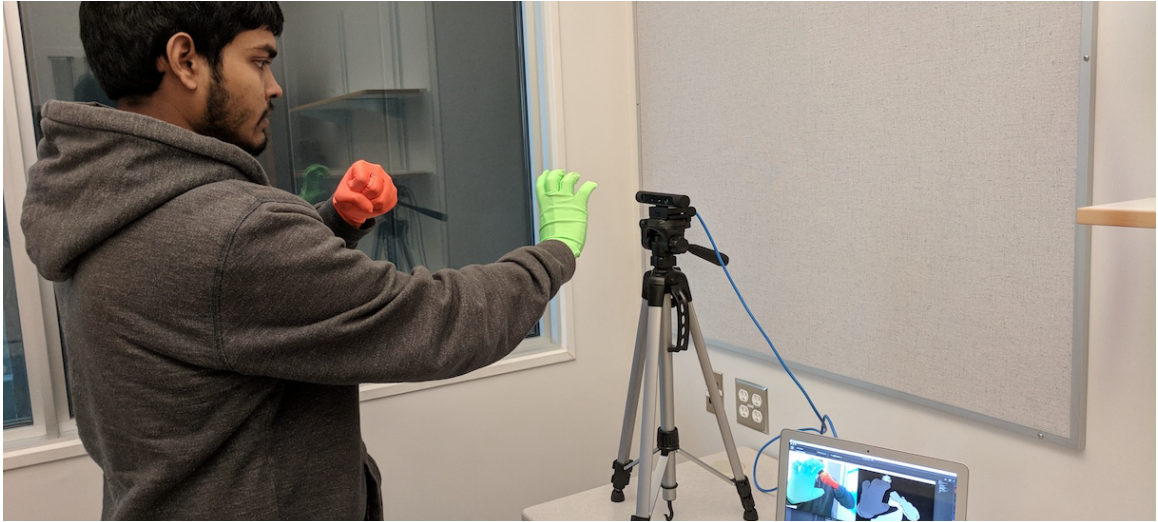
Figure 3.1: Our dataset is generated by recording a subject performing various hand movements wearing a pair of bright colored gloves in front of a RGB-D camera. To the best of our knowledge, our dataset is the first two-hand dataset for hand segmentation.
