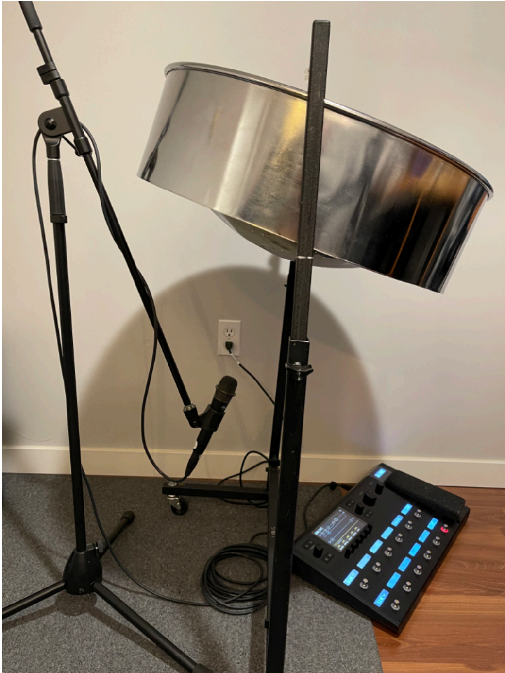
Figure 6.4: Side view of the microphone placement connected to the Line 6 Helix.
