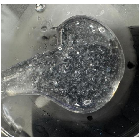
Figure 7: Figure shows KGM gel leachate formed by the action of ECH in a petri dish.
