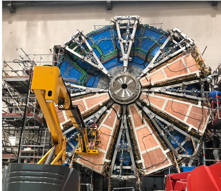
Figure 3.3: NSW C under construction, with 5 out of 8 small sectors installed onto the wheel. The wedge-shaped metal spokes for the small sectors are all present on the Wheel.
