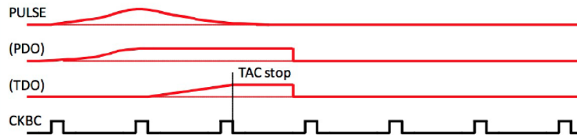
Figure 3.10: Example of pulse and PDO and TAC conversion for a VMM operating in continuous mode [19]. The bunch crossing clock (CKBC) is shown with the time conversion process stopping at the end of a bunch crossing.
