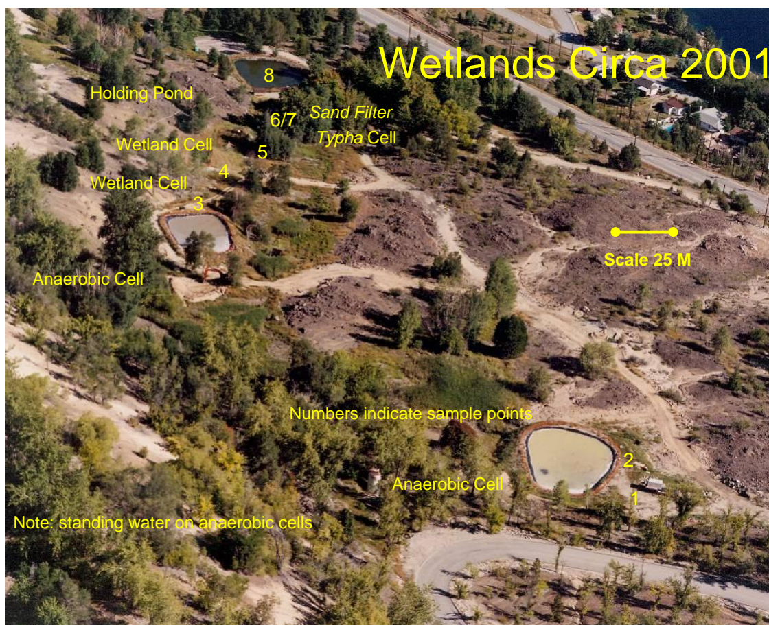
Figure 4. Labelled aerial photograph of wetlands system with sampling points indicated.
