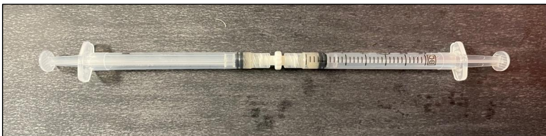
Figure 3.4 Image of double-syringe method for mixing particles and alginate hydrogel
