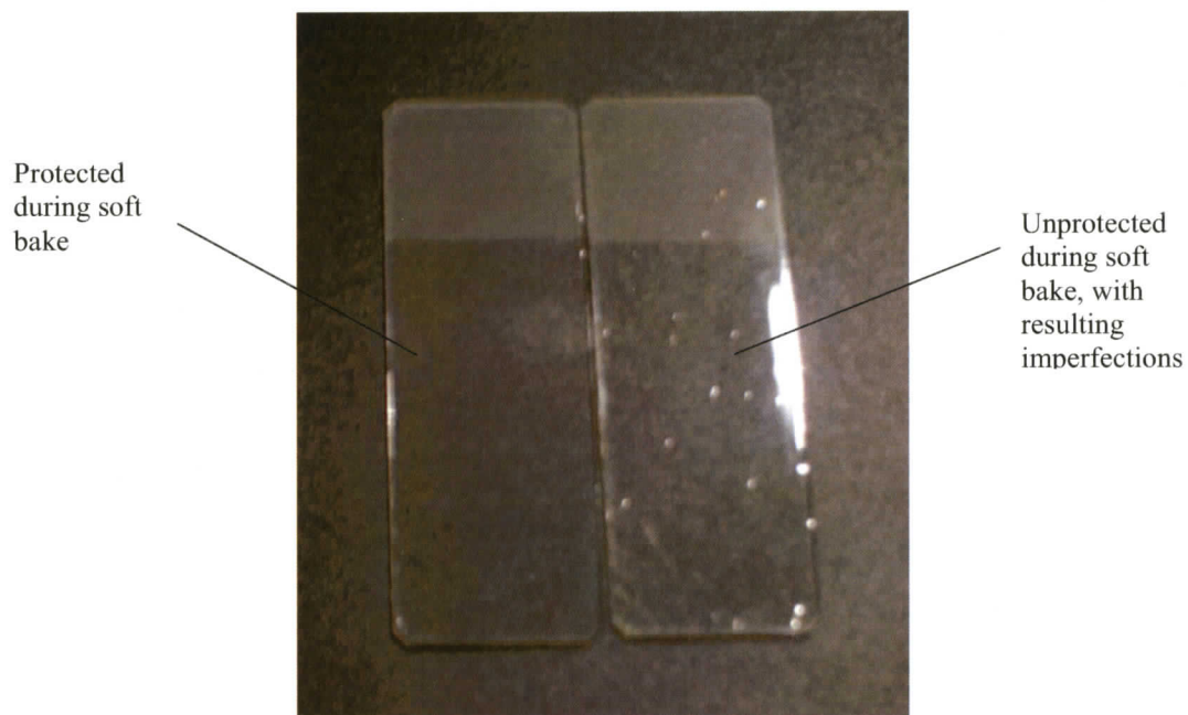
Figure 2.6 Image of photoresist-coated microscope slides. Sample on the left was protected by dust cover during soft bake, while the layer on the right was unprotected and contains a number of surface imperfections.
