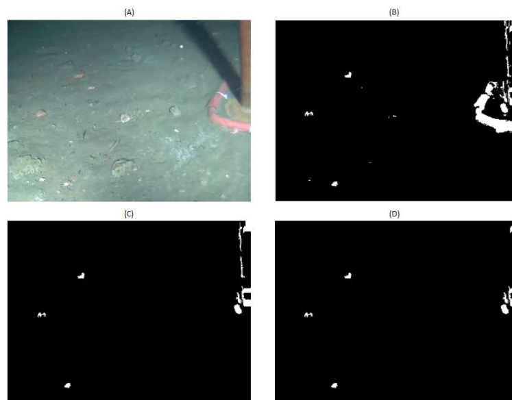
Figure 3.12: Images illustrating the segmentation process in the HSV color space. A) Original image. B) Binary image output by color-based thresholding. C) Image after the elimination of regions with undesirable area range. D) Image after the elimination of regions with undesirable eccentricity values.
