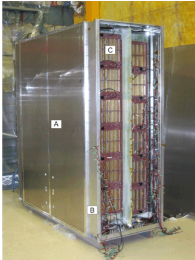
Figure 3.8: TPC outer box. A: one of the outer box walls; B: service spacer; C: one of the Micromegas modules inserted into the module frame [76].
