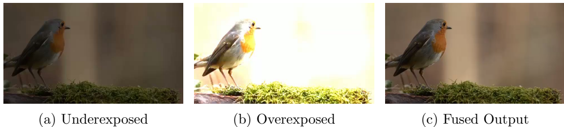
Figure 4.4: Example of multi-exposure video fusion results. (a) Underexposed frame, (b) Overexposed frame, and (c) the fused output produced by the proposed gradient-domain framework. The fused result preserves details from both input exposures while maintaining balanced brightness and temporal consistency.
