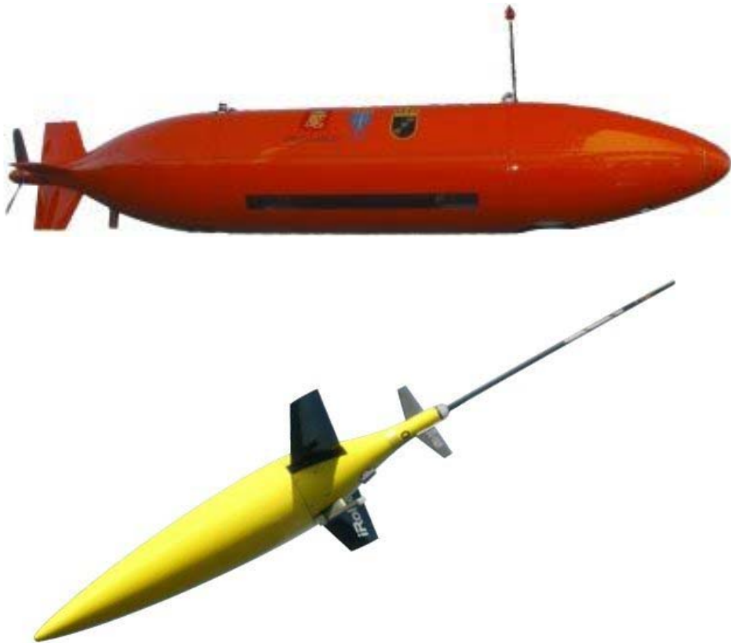
Figure 1-1. Commercial AUV Products. Top: the HUGIN™ AUV manufactured by Kongsberg Maritime uses a single transom mounted thruster for surge propulsion and four individually controlled rudder blades for heading, pitch, and roll control. Bottom: the Seaglider™ manufactured by iRobot varies its buoyancy to glide through the water column over month long missions. Images courtesy of http://auvac.org/resources/configuration .
