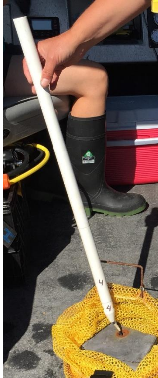
Figure 1: Tilt Current Meters (Lowell Instruments LLC) were deployed in 10 meter depths (below chart datum). These loggers require a large, flat area free of obstructions to move freely.
