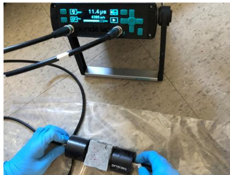
Figure 18: UPV test arrangement for mortar
