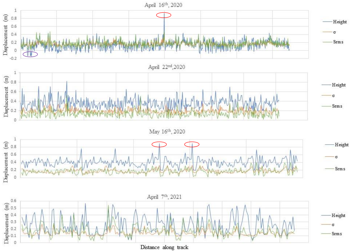
Figure 4.6. Along-track profiles of object-wise mean values of IS-derived surface parameters h , \sigma , S_{rms} during winter 2020 and 2021. The red circle is showing a thicker MYI area. The purple circle is the FYI area between MYI and Stefansson Island. The distance along track is \sim 284.7 km (April 16 th , 2020), \sim 157.3 km (April 22 nd , 2020), \sim 59.61 km (May 16 th , 2020), and \sim 86.93 km (April 7 th , 2021).
