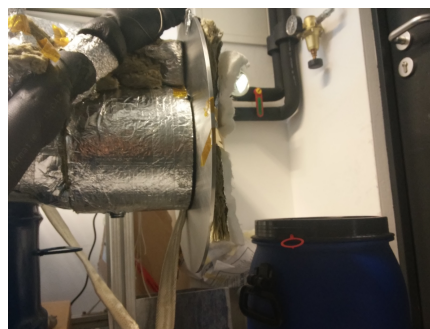
(b) Disc setup with electrical heating tapes after insulation applied.
