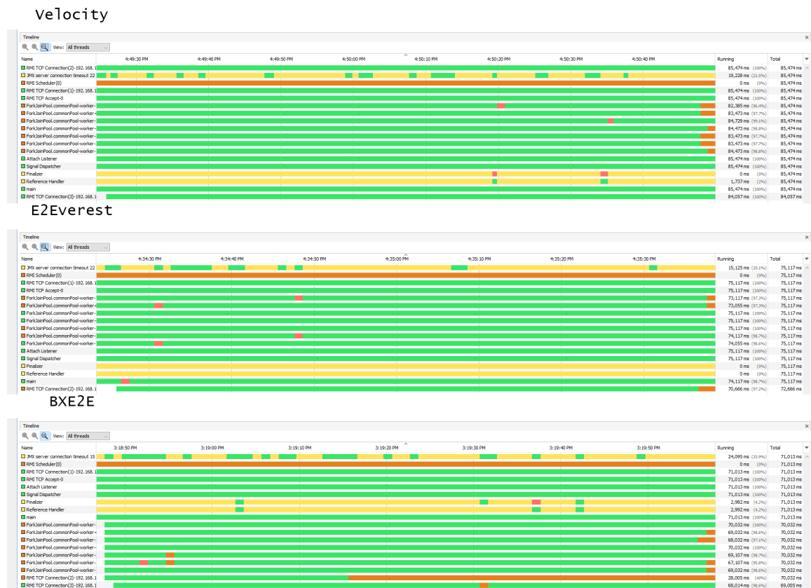
Figure 6.7: Overall thread utilization of the three frameworks with verification
