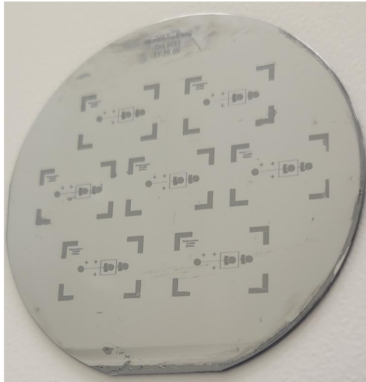
Figure 2-7. The final microchannel mould
