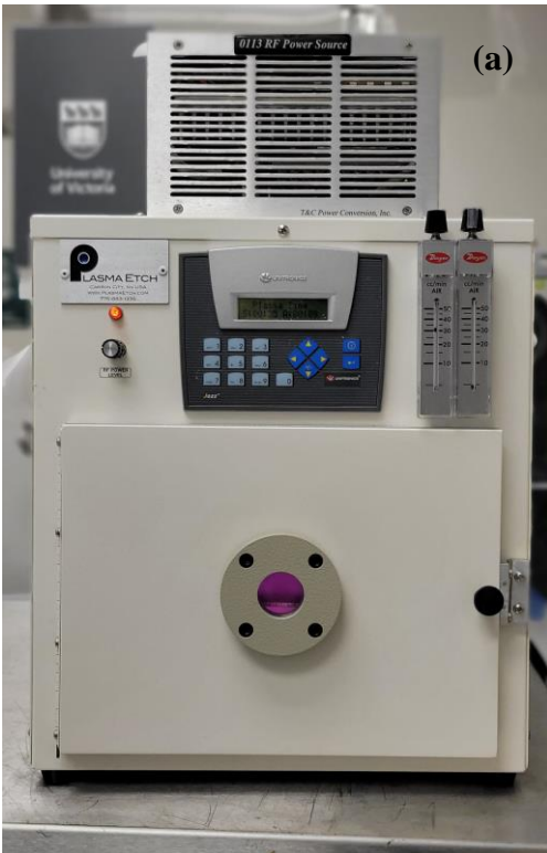
Figure 2-9. (a) Using plasma to bond PDMS and glass. (b) The benchtop aligner
