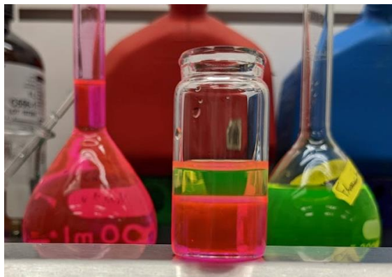
Figure 4-2 Fluorescein dissolved in basic water, layered on top of rhodamine B in glycerol. The stock solutions can be seen in the background of the image.
