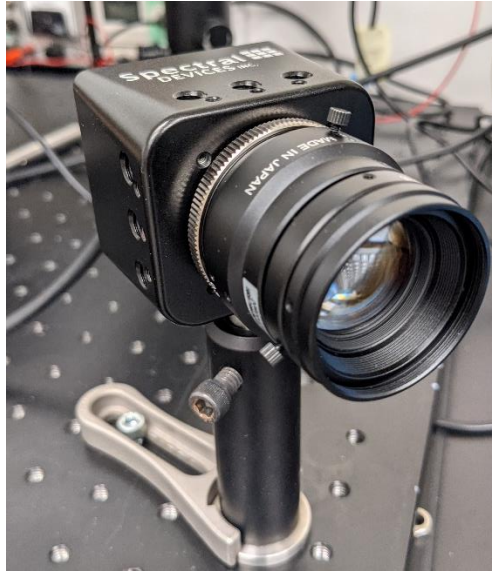
Figure 3-11 Photo of 8-channel visible hyperspectral camera (msCam VIS8, Spectral Devices Inc).
