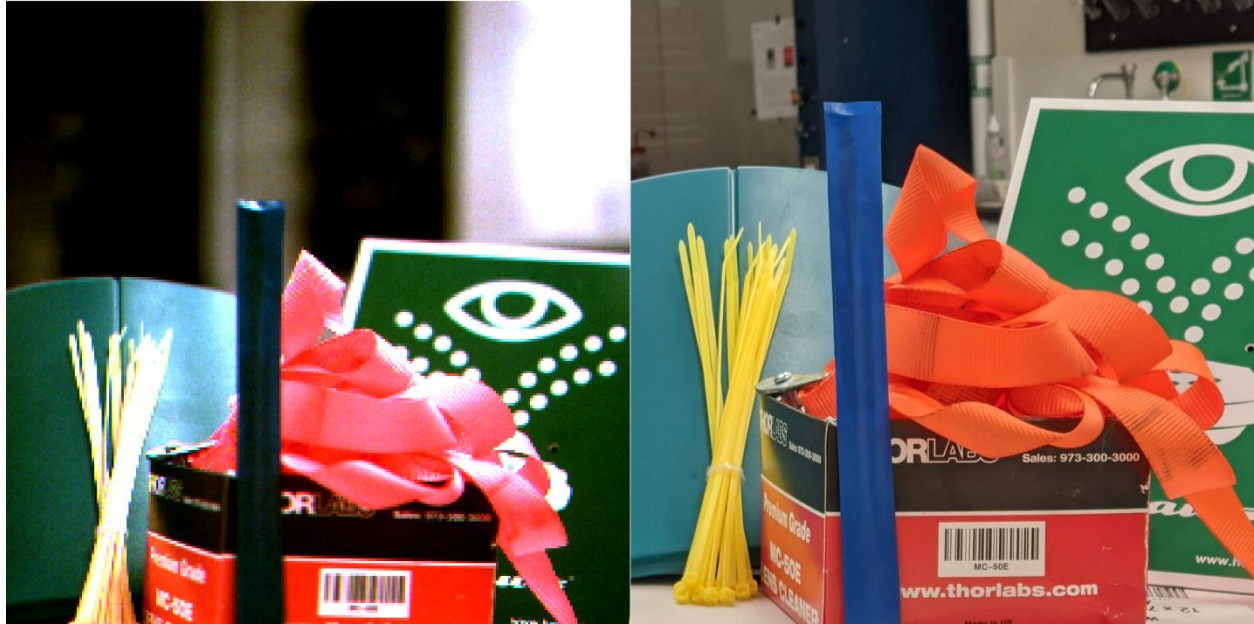
Figure 3-14 False-coloured RGB Image vs Cell Phone Image. RGB image (left) generated from the hyperspectral image in Figure 3-13. The red, green, and blue values are assigned from the intensities of the 640 nm, 526 nm, and 474 nm hyperspectral channels, respectively. Cell phone image of the same assorted materials (right).
