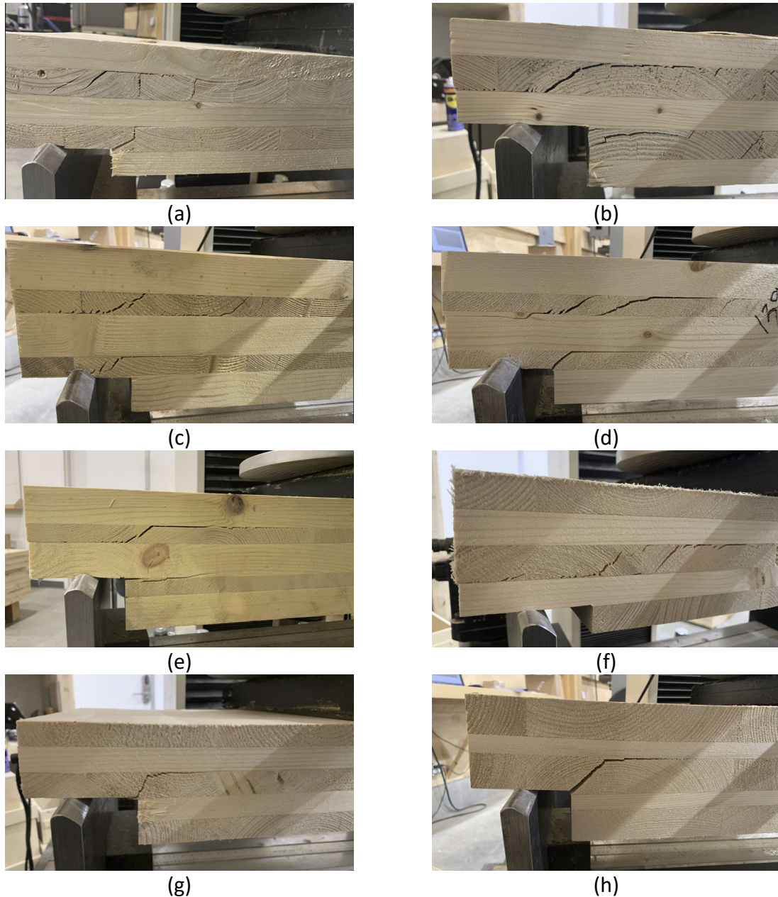
Figure 14: Rolling shear-notch failure mode of reinforced specimens; (a) 100 ||-20-R, (b) 100 ||-40-R, (c) 139 ||-35-R, (d) 139 ||-35-IR, and (e) 139 ||-52-R, and rolling shear failure mode of (f) 100 ⊥-20-R, (g) 100 ⊥-40-R, and (h) 139 ⊥-52-R.
