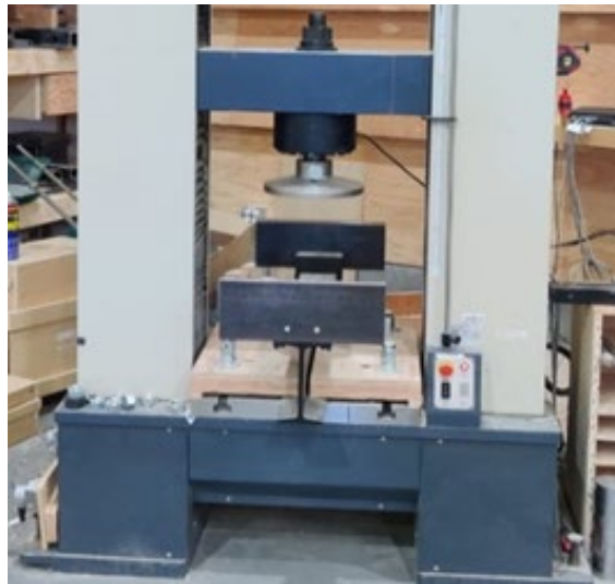
Figure 3: Test setup: Universal Testing Machine.
