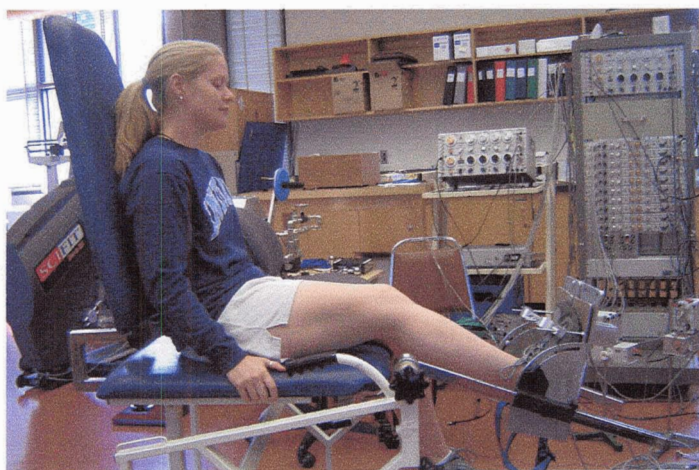
Figure 2. Experimental setup during isometric plantar flexion.
