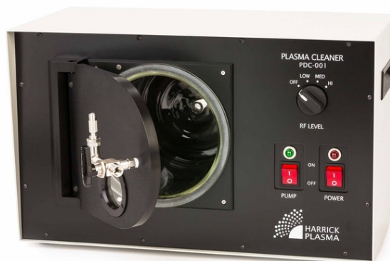
Figure 4.2: Harrick PDC plasma cleaner used for surface etching.
