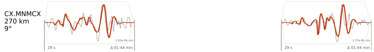
Figure B.8: Observed (grey) and synthetic (red) waveforms of radial, transverse, and vertical components (R, T, and Z, respectively). The shading around the red seismograms is composed of 100 random synthetic seismograms drawn from the posterior probability density. Labels on the left are network code, station code, epicentral distance and azimuth. Labels within the plots are window start time after centroid time (left), window duration (bottom right) and amplitude (top right).
