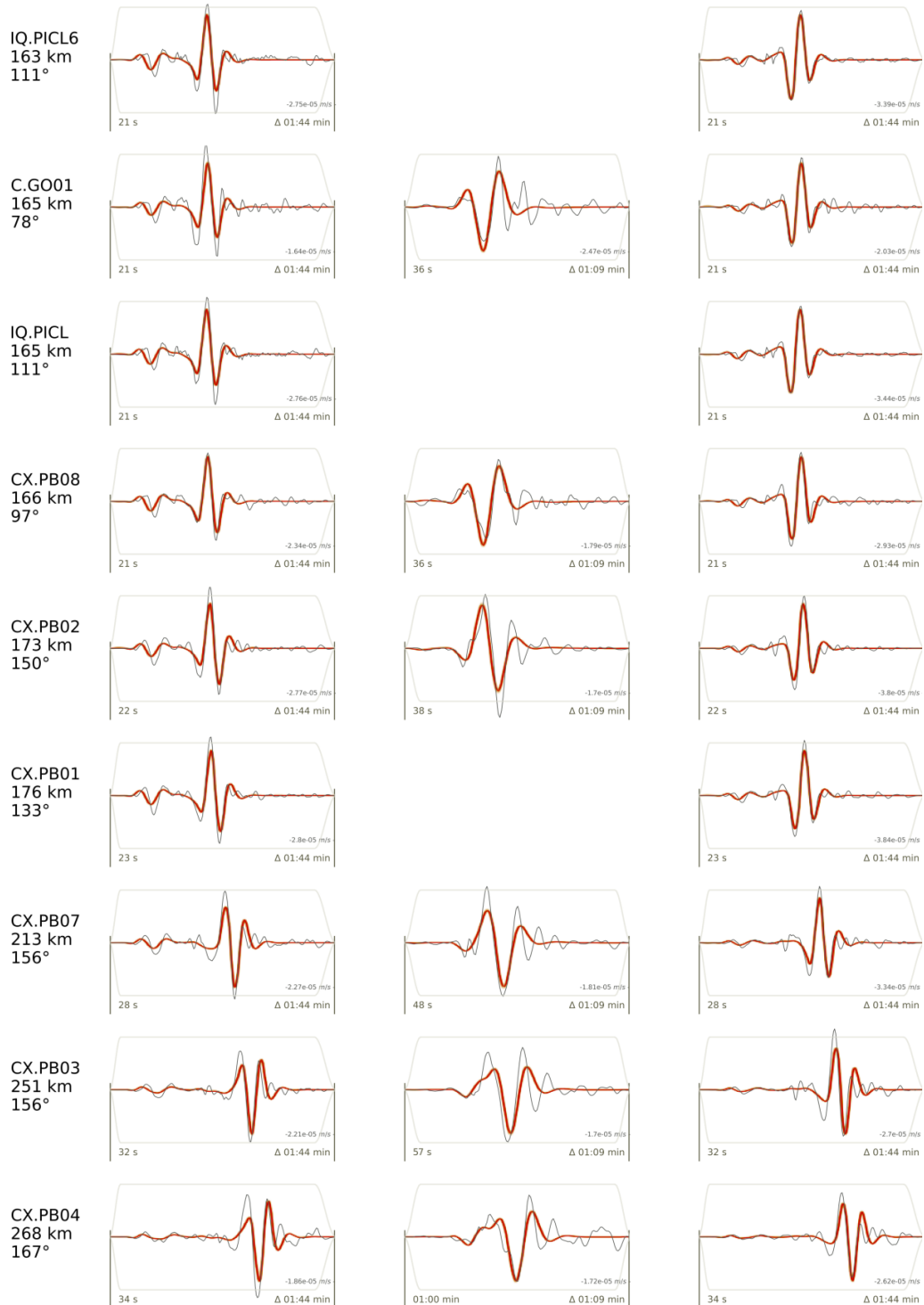
Figure B.12: Observed (grey) and synthetic (red) waveforms of radial, transverse, and vertical components (R, T, and Z, respectively). The shading around the red seismograms is composed of 100 random synthetic seismograms drawn from the posterior probability density. Labels on the left are network code, station code, epicentral distance and azimuth. Labels within the plots are window start time after centroid time (left), window duration (bottom right) and amplitude (top right).
