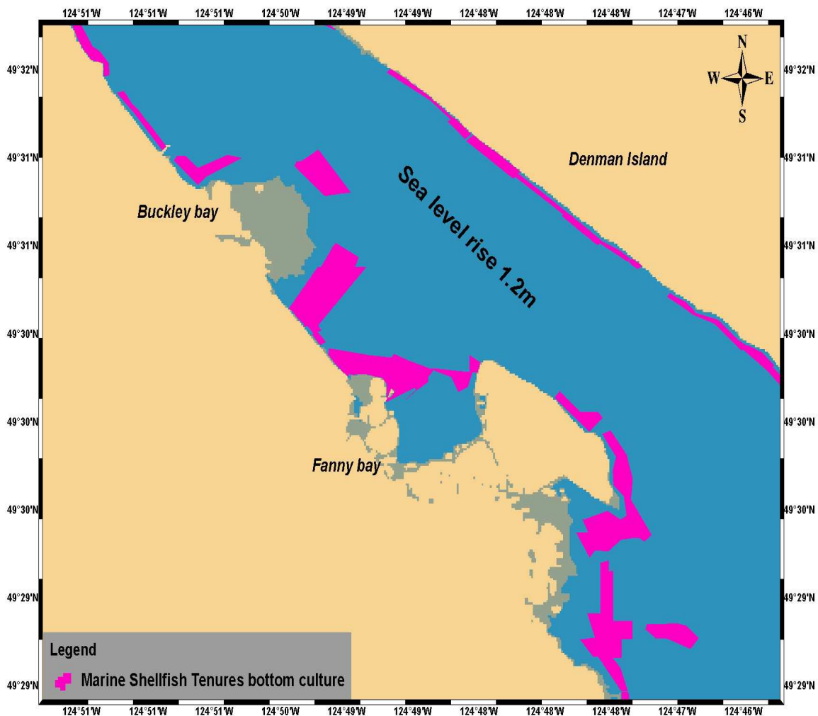
Figure 16: Simulation of 1.2 metre SLR in Buckley bay and Fanny bay (1:25,000)
