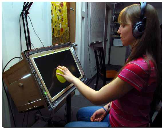
Figure 4.1: A participant about to perform a grab action on the prototype interface. Once the action is performed the yellow circular object will fade away and the target will be highlighted. A short distinct sound is given after the participant performs either the grab or release action.
