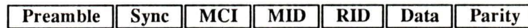
Figure 3.2.4 Transmit Segment Format as used in a Meteor Burst Data Acquisition Network
