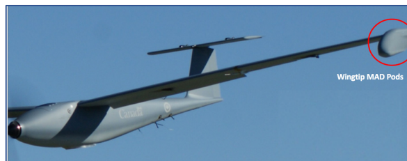
Figure 3: Brican TD100 UAV: Wingtip MAD Pods Annotated (Modified from [10])
