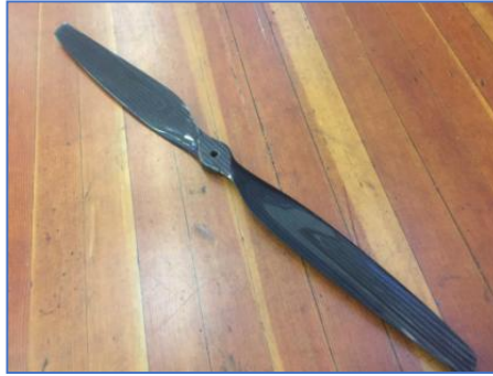
Figure 62: VTOL Carbon Fiber Propeller
