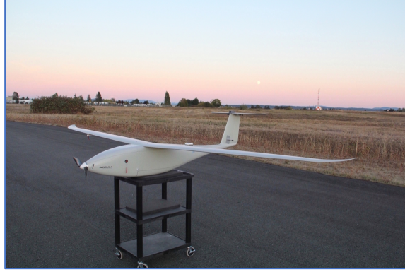
Figure 5: Nebula N1 UAV: Conventional Configuration [14]
