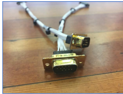
Figure 58: DGPS to Aft Switchboard Connector
