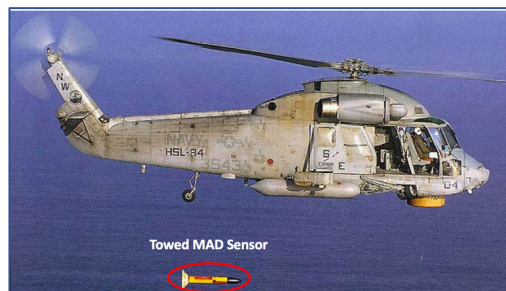
Figure 2: SH-2G Super Seasprite ASW Helicopter: Towed MAD Annotated (Modified from [6])
