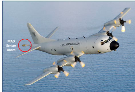
Figure 1: P3 Orion ASW Aircraft: MAD Boom Annotated (Modified from [5])
