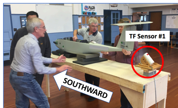
Figure 48: Fuselage Unpowered Static Field Pull-Away Test: Translation Southward
