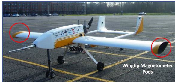
Figure 4: Carleton-Sander GeoSurv II UAV: Wingtip Magnetometer Pods Annotated (Modified from [11])
