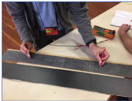
Figure 63: Resistance Test on Carbon Fiber Skin Sample
