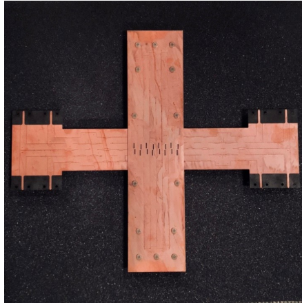
Figure 4.4: Manufactured 1-dimensional beamforming prototype.
