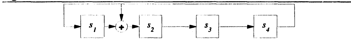
Figure 6.1 Internal LFSR for x^4 + x + 1
