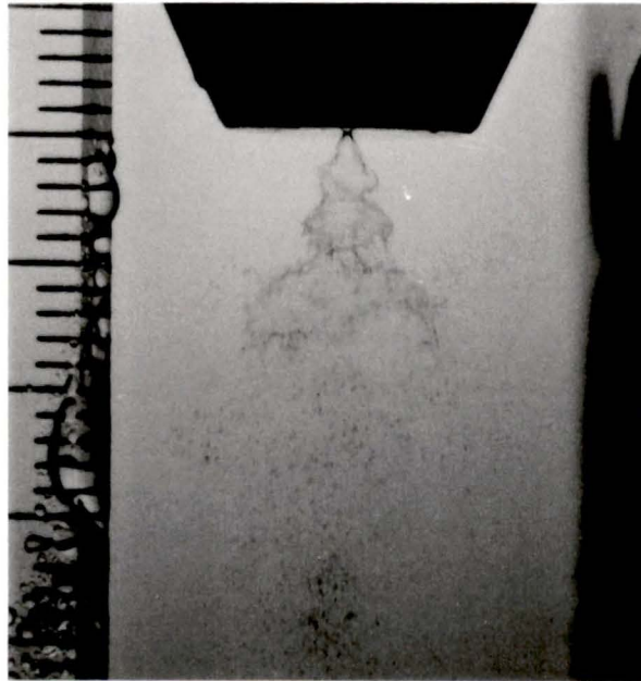
Figure 5.8: Photograph of the spray produced by the modified pressure-swirl atomizer with Insert # 3 with acoustic excitations. p = 0.4 MPa (60 psi), f_a = 240 Hz, power level 4.
