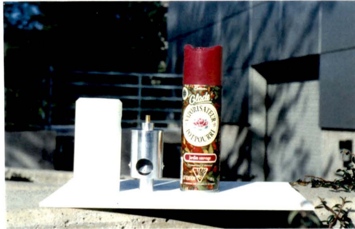
Figure 6.9: Photograph of the prototype design of the new-concept impaction atomizer.
