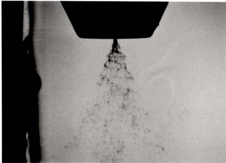
Figure 5.12: Photograph of the spray produced by the modified pressure-swirl atomizer with acoustic excitations. p = 0.4 MPa (60 psi), f_a = 1 kHz, power level 3.
