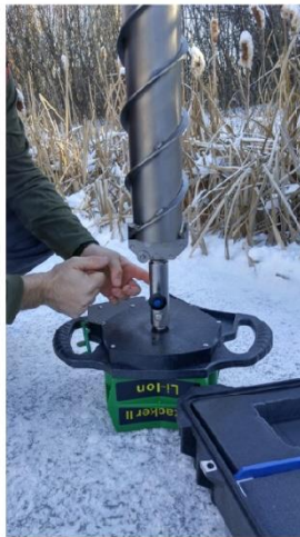
Figure 3 Attach auger tube to sleeve and connect using pin
