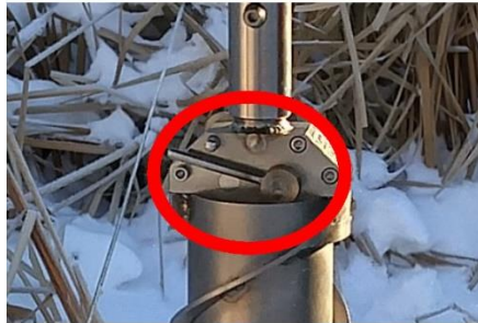
Figure 6 Remove motor and auger head by moving switch, shown in red circle
