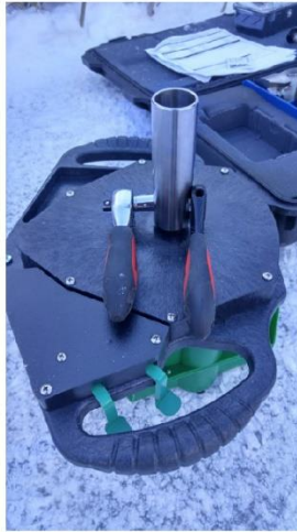
Figure 2 Attach sleeve to auger motor with bolt and nut
