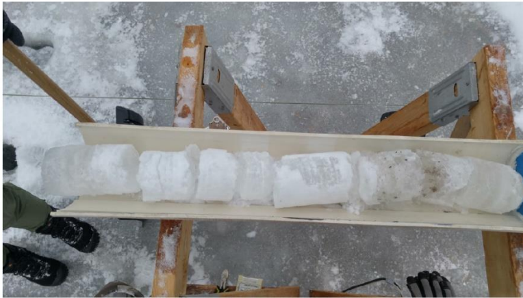
Figure 1 Ice core catching device example set-up
