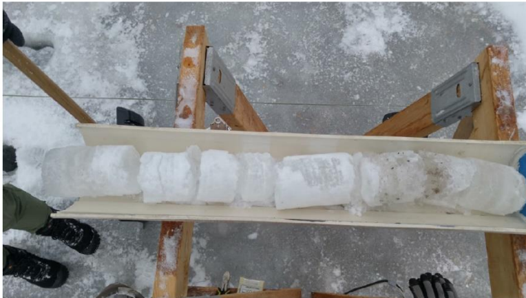
Figure 1 Ice core catching device example set-up
