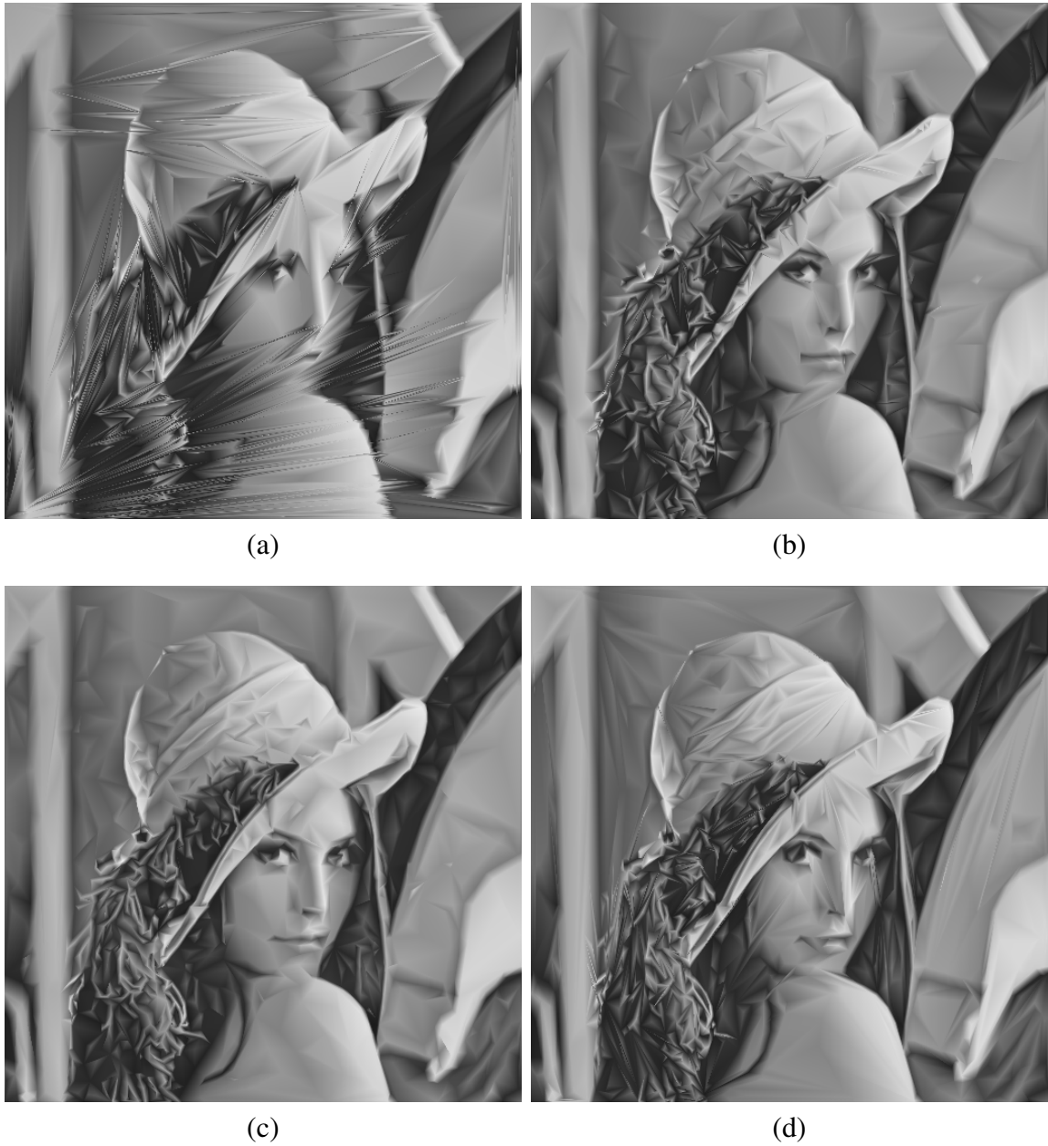
Figure 3.10: Comparison of the mesh quality obtained for the lena image at a sampling density of 1% with various main edge-flip criteria (Cont'd) (a) DP (22.75 dB), (b) ELABN (27.17 dB), (c) ELJND (28.58 dB), and (d) YMS (27.19 dB).
