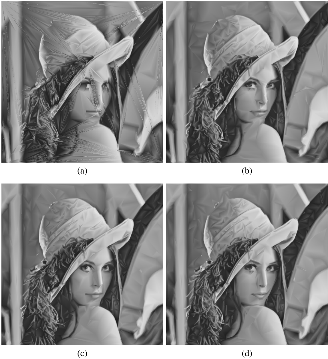
Figure 3.11: Comparison of the mesh quality obtained for the lena image at a sampling density of 1% with various main edge-flip criteria (Cont'd) (a) SE (24.20 dB), (b) GHH (28.93 dB), (c) SQSE (29.41 dB), and (d) JNDSE (29.41 dB).
