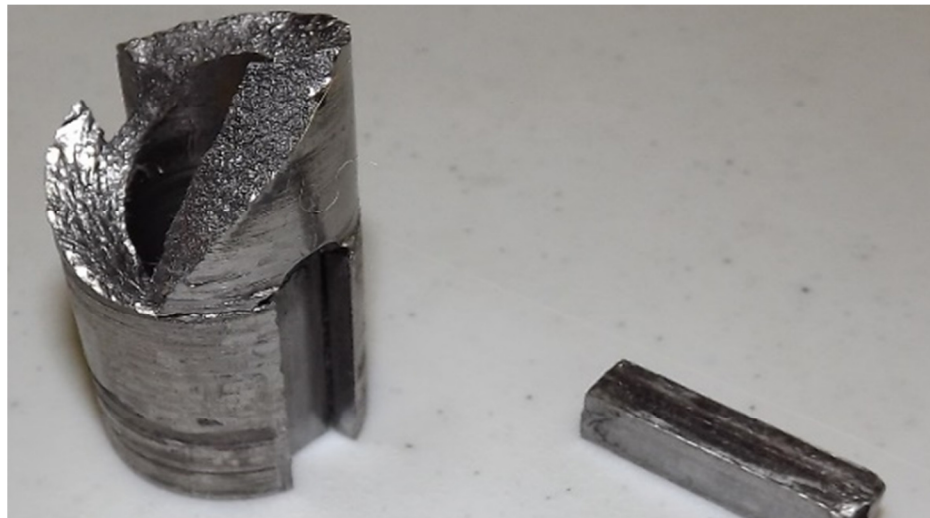
Figure 74: Broken Crankshaft Snout and Sheared Key
