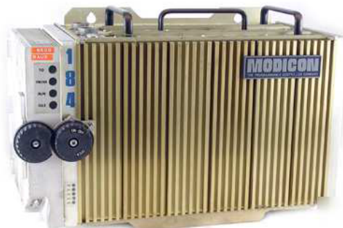
Figure 1.3: The Modicon 184, second generation of PLC designed by Modicon [1]
