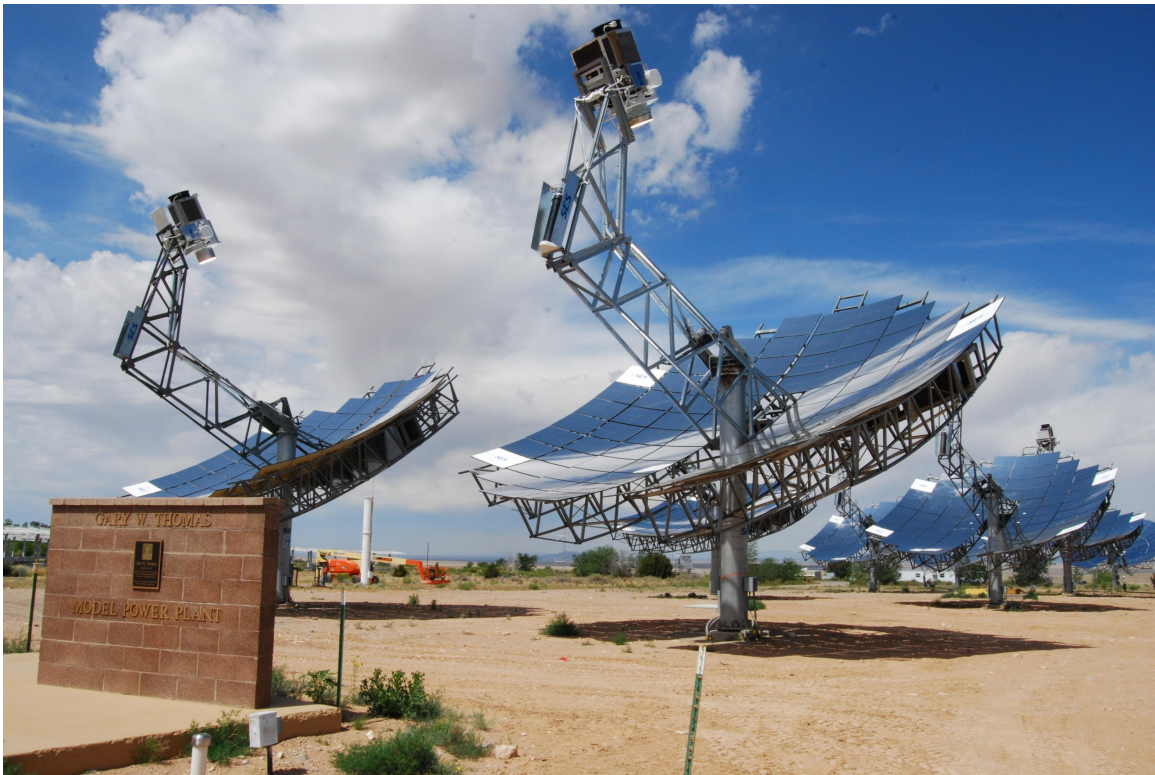
Figure 1.8: A stirling solar engine in Sandia National Laboratories, Albuquerque, New Mexico.
