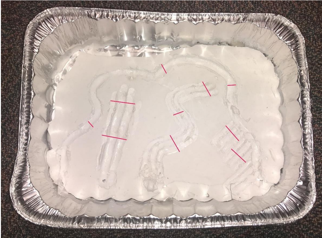
Figure 23. Plaster panel 2 with marked measurement locations.
