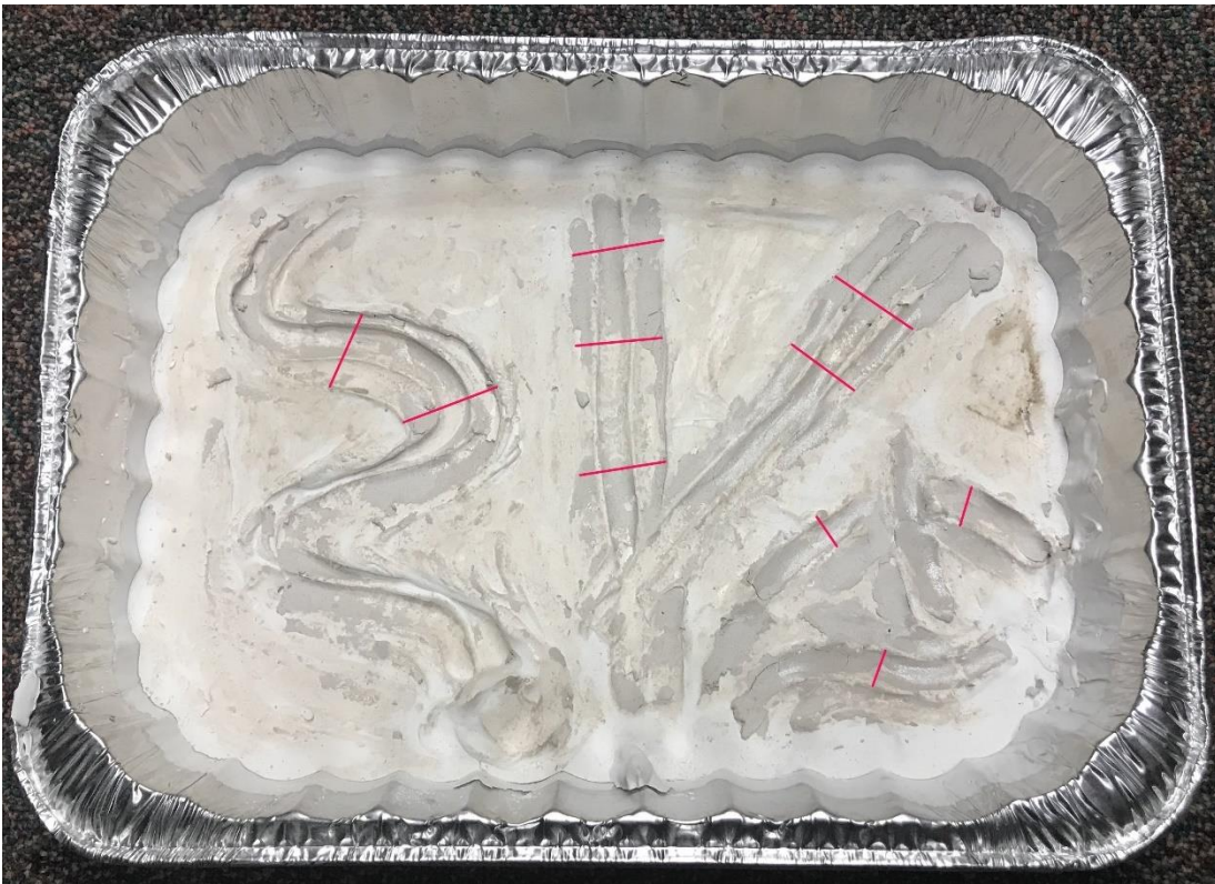
Figure 30. Plaster with clay panel 3 with marked measurement locations.
