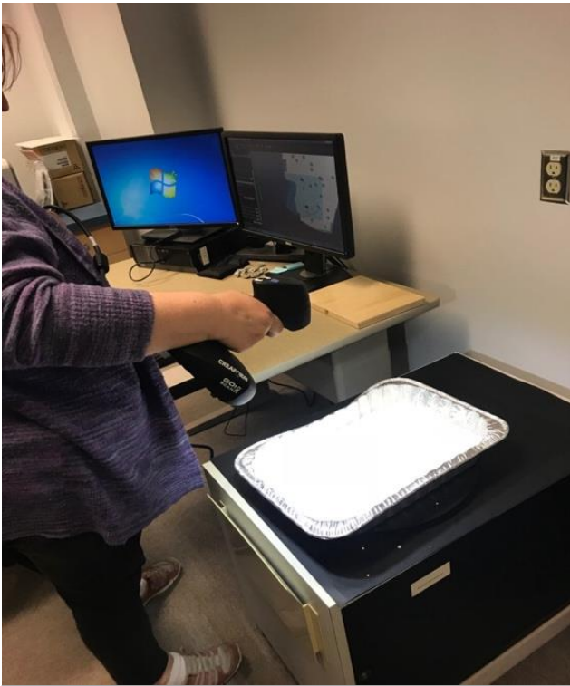
Figure 4.11: Handheld structured light scanner set up.
