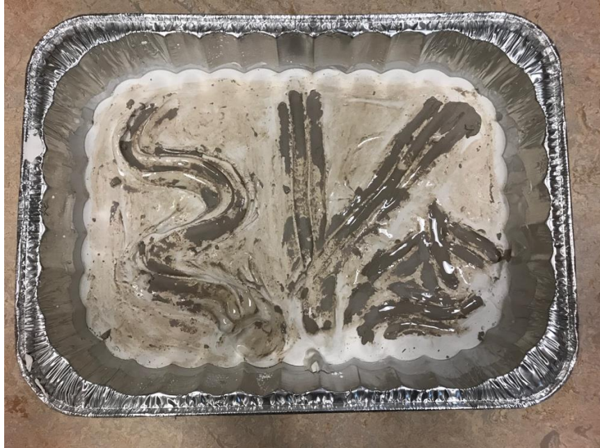
Figure 4.8: Plaster panel with clay and gloss.
