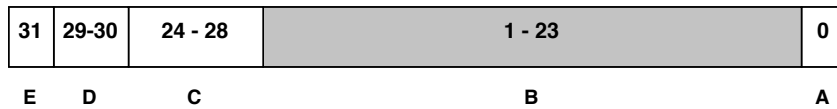
Figure 6.2: Bit regions making up the LATCH variable. In order to index the phase space beamlet numbers are assigned to each particle in the shaded bit region (B). By writing the beamlet numbers into the LATCH variable, the particles of each beamlet and all associated secondary particles can be tracked throughout a simulation.
