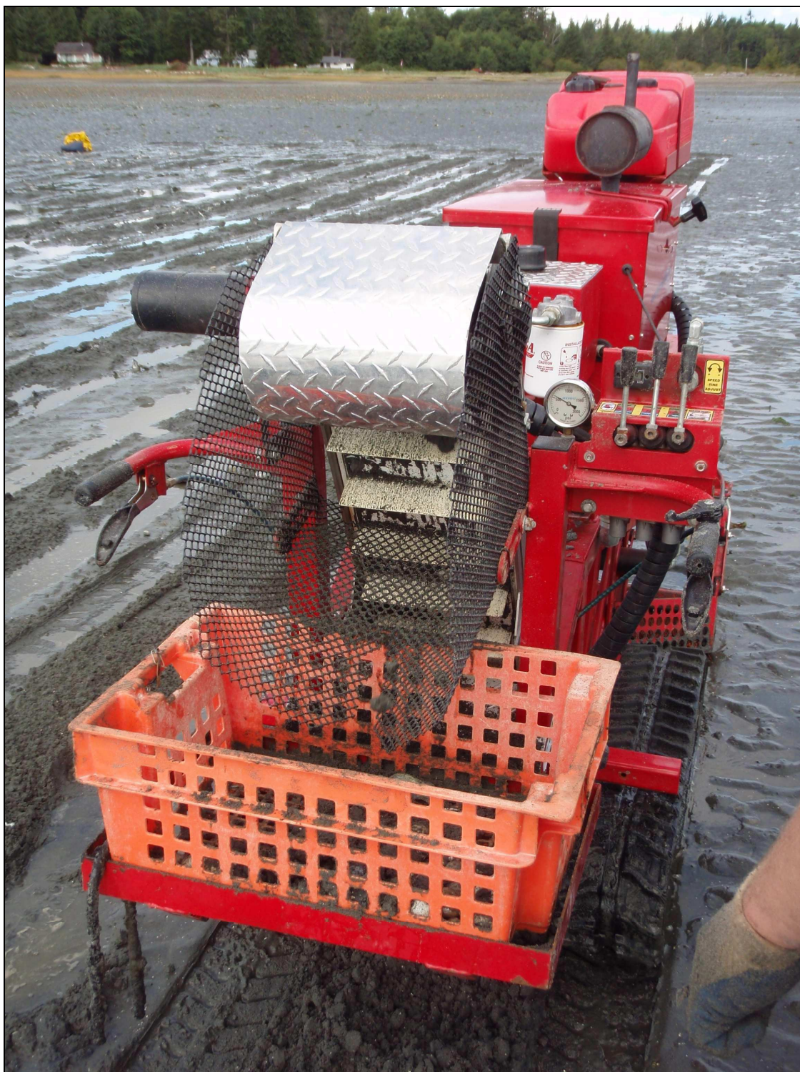
Figure 8. Operator view of prototype mechanical shellfish harvester
