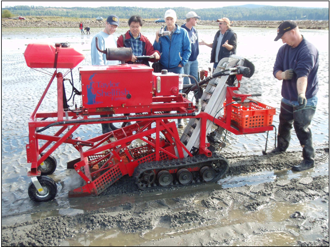
Figure 7. Side view of prototype mechanical shellfish harvester
