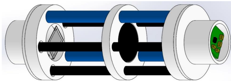
Figure 3.16 SolidWorks assembly of the prototype#1 ISDS sensor head.
