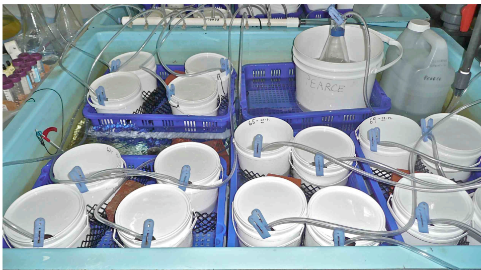
Figure 7. Photo of seawater table with 16 aerated containers for temperature/diet experiments (12 for experiments and 4 as part of wet/dry weight comparisons)
