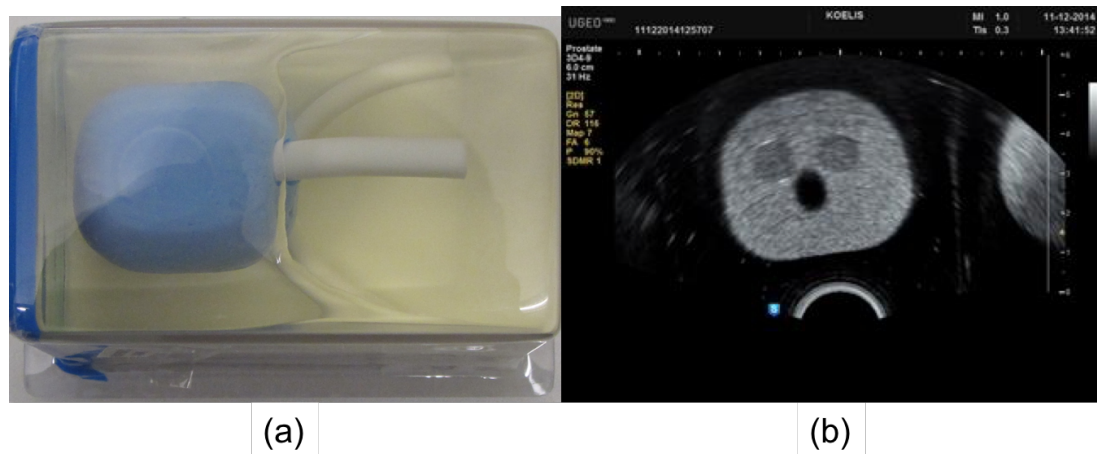
Figure 3.2 CIR phantom model 053L: (a) phantom in the container, (b) The conventional ultrasound image of the phantom [48].
