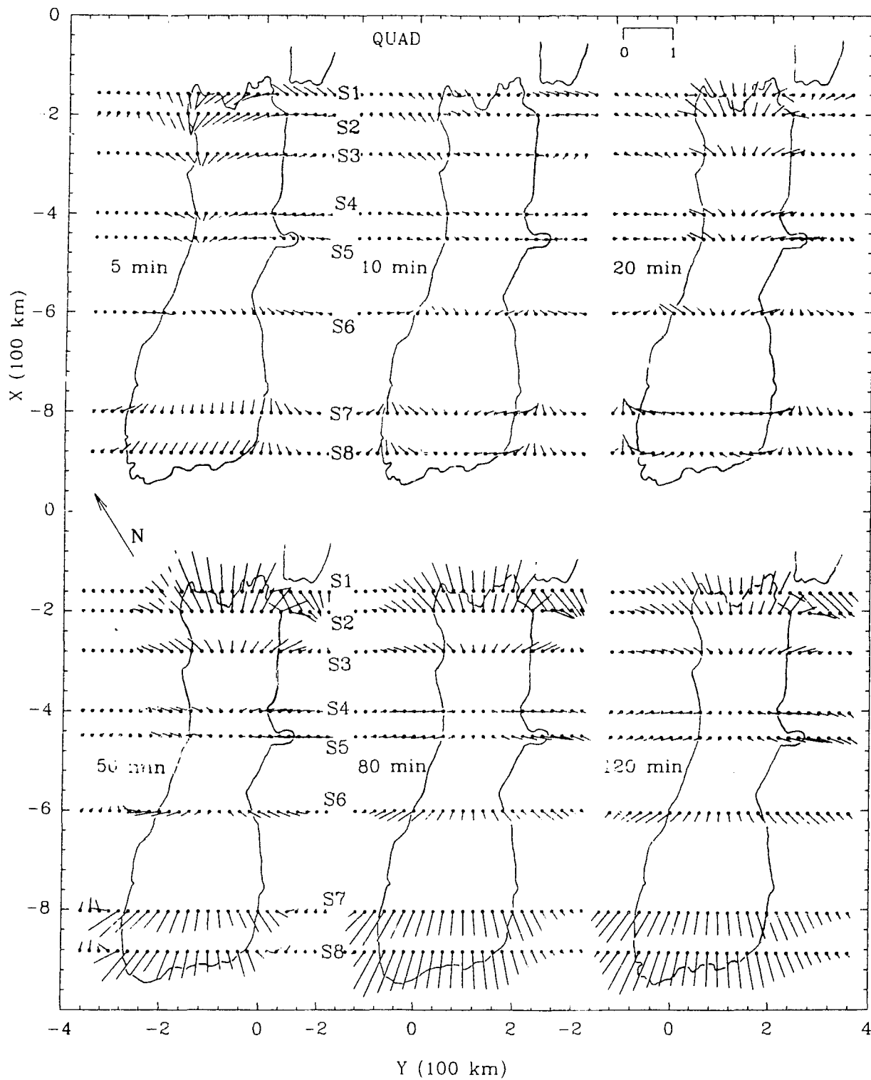
Figure 6.11: The quadrature induction arrows for traverses S1-S8 on South Island for periods of 5-120 min.
