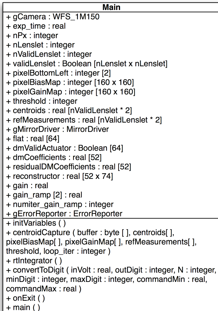
Figure 43: The UML representation of the pipeline main ( ) program.
