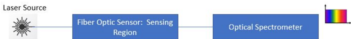
Figure 1.5: Spectrometer reads the signal from the sensor and displays the signals on GUI to analyse the sample
