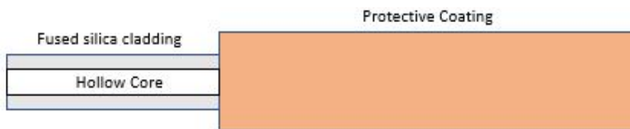
Figure 1.4: Hollow core fiber with fused silica cladding and polyamide protective coating
