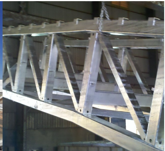
(d) Galvanizing of truss for Ford Pedestrian Bridge, Chicago, IL, United States
