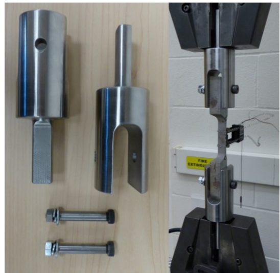
Figure 11: Testing of corner coupons with special grips and pins
